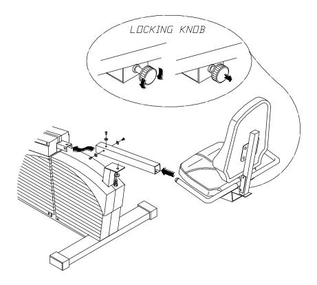
**6.** Slide seat carriage onto seat carriage tube and secure with cam lock as pictured above.
